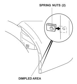
Position the rear splash guard on the rear bumper and fenderwell, and install three self-tapping screws.
