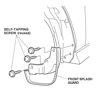
Turn the steering all the way clockwise and repeat steps 2 and 3 to install the right front splash guard.
