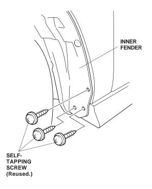
3. Position the front splash guard on the inner fender, and reinstall the three self-tapping screws.
