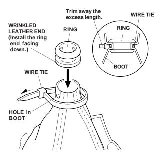
Secure the boot to the ring with the wire tie as shown.
