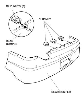
9. Slide the two spring nuts (one on each side) over the dimpled areas of the rear bumper.
