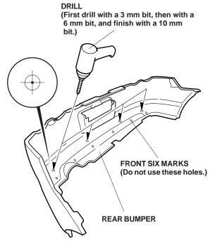
4. Position the template on the inside of the rear bumper, and align its curved edge with the root of the arch on the rear bumper.
