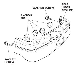
14. Reinstall the rear bumper. Install the two long washer-screws from the kit in the lower holes in the wheelwell area. Check that the clips and other fasteners are installed securely without play or lifting. 15. While holding light pressure on the rear under spoiler, slowly and carefully remove the adhesive backings. Hold the under spoiler firmly against the rear bumper with the palm of your hand while holding the rear bumper with the palm of your other hand in the opposite direction.
