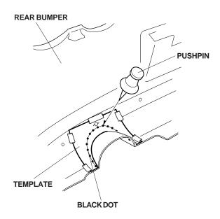
5. Using a pushpin, make a series of holes through the rear bumper along the line shown on the template.
