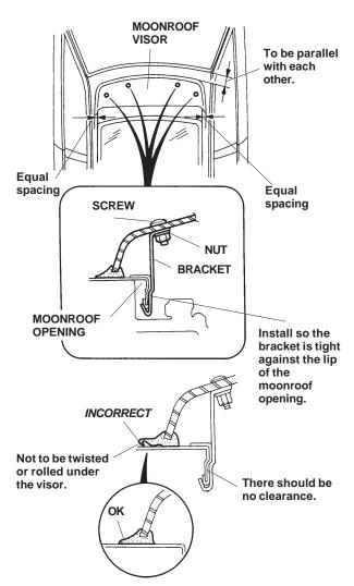
11. Tighten the nuts and screws, alternating between sides. To prevent damage to the resin nuts, do not overtighten the screws.
