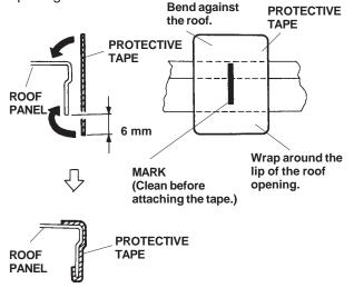
8. Place the two front brackets A into position by sliding them along the lip of the roof opening. Set the moonroof visor on the vehicle's roof, forward of the moonroof opening, and adjust its position so the holes in the visor are aligned with the protective tapes.
