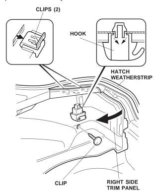
Insert one bolt from the kit into the clip hole indicated, then install a nut on the end of the bolt. Tighten the nut securely.
