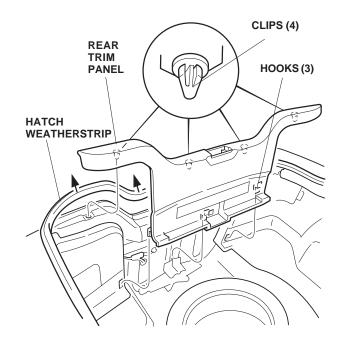
3. Remove the hatch weatherstrip in the area shown, then remove the three clips and one hook that secure the right side trim panel. Gently fold the panel out of the way.
