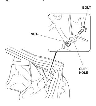
5. Reinstall the right side trim panel, then thread the hook from the kit onto the bolt you just installed.
