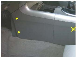
6. Unplug the power connector (rear cig. Lighter) and lift the console out of the area.
