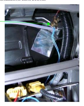
4. OK, give it a test. Make sure your rear defroster works and the heated mirrors too (both sides). If so, check and make sure all the plugs and connectors you undid are reconnected. Put the Dash panel back and the center console.
