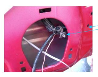
Release the wire ties to get some slack on the wiring harness
