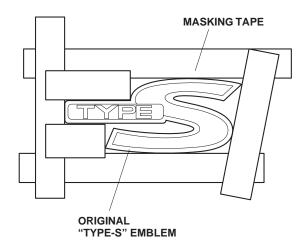
2. Remove the original "TYPE-S" emblem by cutting around the outer edges with a piece of string as shown.
