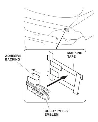
5. Remove the masking tape from the trunk lid.
