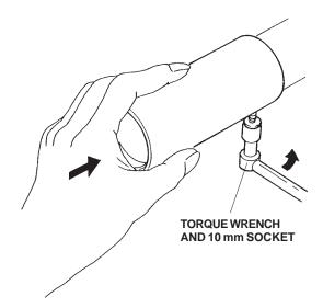
5. Start the engine, and rev it up a few times. Listen for any rattling noise coming from the exhaust pipe finisher, and adjust as necessary.
