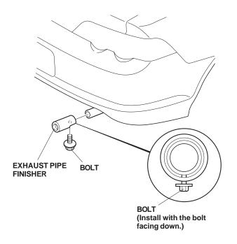
With the bolt facing down, slide the exhaust pipe finisher onto the exhaust pipe until it bottoms against the exhaust pipe.
