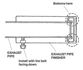
4. While pushing the exhaust pipe finisher firmly against the exhaust pipe, torque the 6 mm bolt to 7 to 12 Nom (5 to 8 lb-ft).
