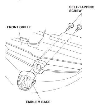
Using diagonal cutters, cut the locating tabs from the existing front "A" emblem. Push the locating tabs to remove the emblem from the emblem base.
