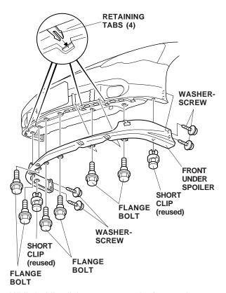
6. While holding light pressure on the front under spoiler, slowly and carefully remove the adhesive backings from the front under spoiler in the direction shown. Press on the front under spoiler with the palm of your hand for 30 seconds.
