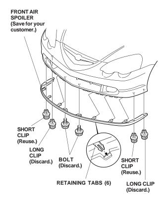
Remove the two self-tapping screws from the front bumper. Slide the four spring nuts (two on each side) over the dimpled areas of the front bumper. Install two short expansion clips (from the kit) in the holes on both sides of the front bumper, then slide the four clip nuts onto the bottom flange of the front bumper through the cutouts.
