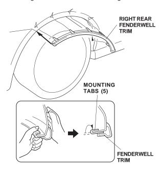
9. Lubricate the inner protector with soapy water, then drive it over the fender flange and fenderwell trim using a rubber mallet.
