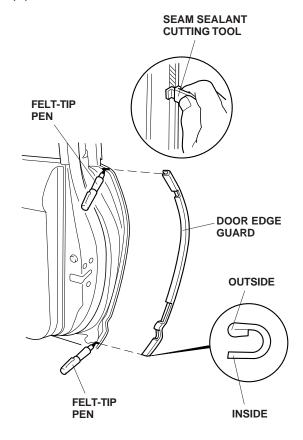
4. Position the cutting edge of the seam sealant cutting tool against the door edge, and trim the seam sealant from mark to mark.
