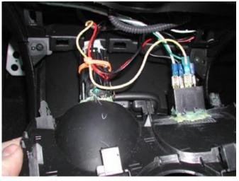
6. Install the relay next to the start for ease of reach. Again i used epoxy.
