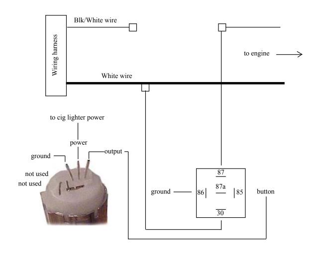
The wiring harness is located in the steering column right next to the ignition switch. Remove the 3 screws from under the dash to access it.
