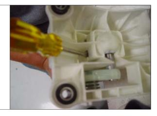
STEP 21. Remove entire shifter stick assembly from the shifter base.
