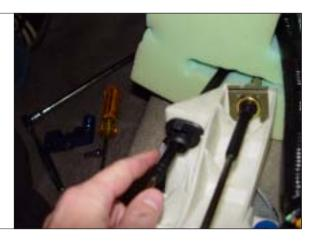
STEP 33. Tighten and secure the shifter housing with the (4) stock bolts and (4) **B&M** solid shifter bushings.
