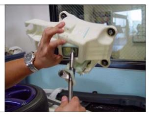
STEP 22. Split the white spherical ball with a flat-head screwdriver and separate into 2 pieces.
