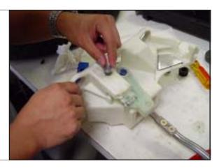
STEP 30. Re-install the shifter assembly and the (4) B&M shifter bushings ①. Re-install wiring harness back into the shifter housing tab.
