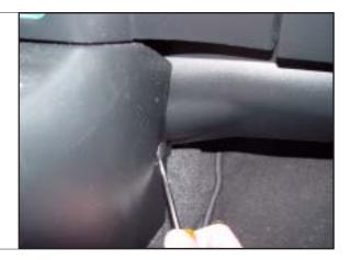
STEP 42\*\*. Re-install the (2) front center console screws.
