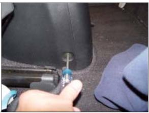
**STEP 10.** Pull up center console to access shift boot retainer.
