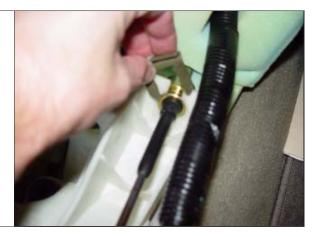
STEP 32. Re-install and secure the cam-style shifter clip.
