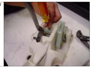
STEP 20. Insert another flathead screwdriver from the underside of the shifter to ease removal.
