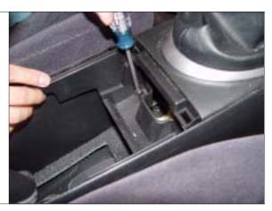
STEP 8\*\*. Pry out (2) screw covers and remove the (2)
