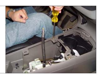
STEP 4\*. Remove the upper center console piece and unplug the electrical connector.
