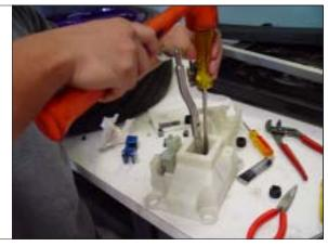
**STEP 29.** Re-install the original shoulder pin into the shifter assembly.
