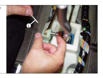
STEP 35. Insert the M8 shoulder bolt through the cable
