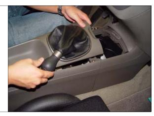
STEP 48. Re-install the shift knob. Test the movement through each gear to make sure shifter engages safely into each gear.
