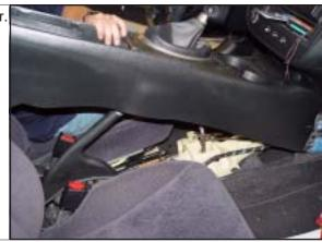
STEP 11. Cut off tie-strap to remove the shift boot from the
