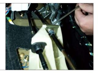
Rotate the cam-style cable clip 90° counter-clockwise and remove. **STEP 14.**
