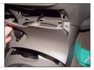
STEP 46\*. Re-install the center console, kick panels, and plug the wire connectors back together.
