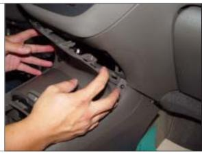
**STEP \*5.** Remove the (2) center console screws.
