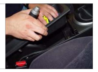
**STEP 7\*\*.** Remove the (2) center console screws.
