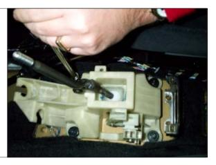
Pull up and remove entire shifter housing. **STEP 17.**
