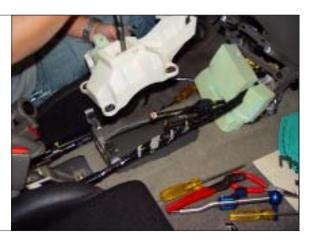
STEP 18. Carefully pry out shifter pin without breaking the plastic shifter housing.
