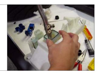
STEP 27. Insert the B&M retainer (G) on top of the stock plastic pivot. Seat the two flat retainer tabs into stock shifter housing first.
