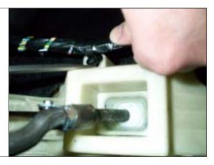
**STEP 16.** Remove the (4) shifter housing bolts.
