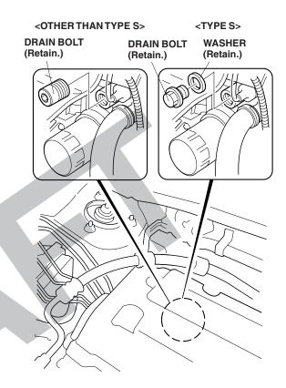
6. Install the new aluminum washer and the engine block heater into the bolt hole using a 24 mm socket and a torque wrench. Torque the engine block heater to 60 N·m (44 lb-ft).
