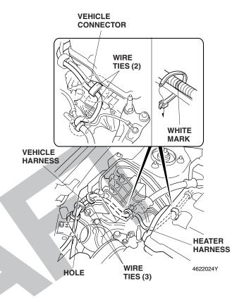
10. Secure the heater harness to the vehicle harness with five wire ties as shown.
