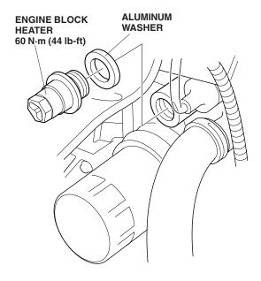
7. Plug the connector end of the heater harness into the engine block heater. Secure the heater harness to the vehicle harness with two wire ties in the areas shown.
