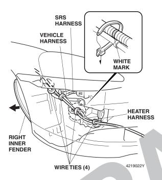
12. Continue routing the heater harness toward the middle of the front bumper, and secure it to the grille with the four wire ties.
